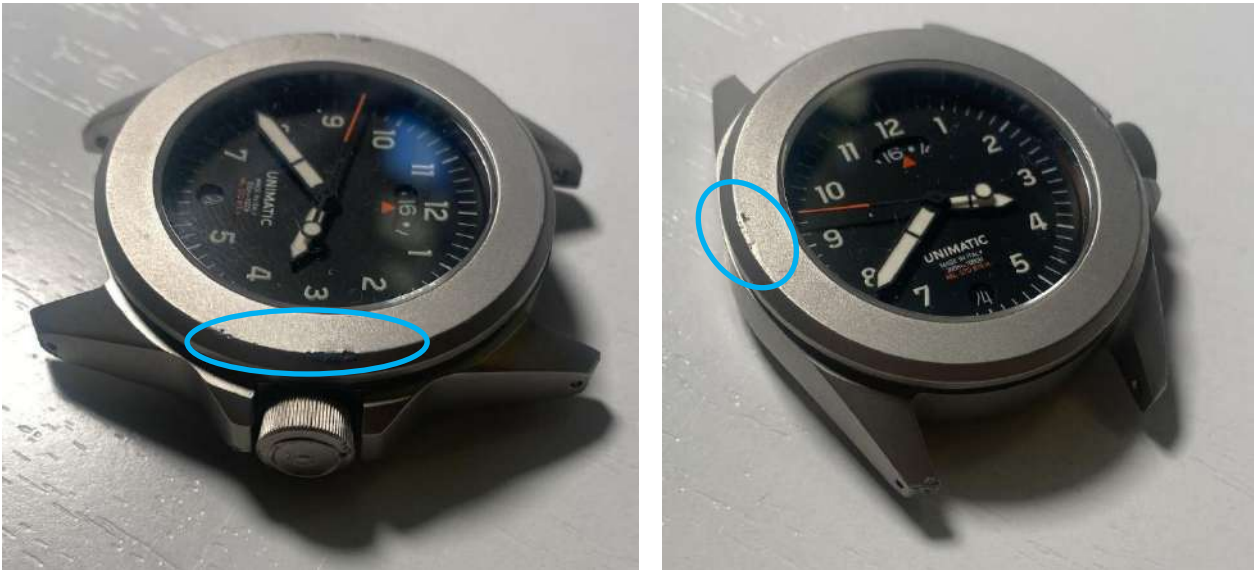
Figure 4 – Example of dents caused by the impacts
