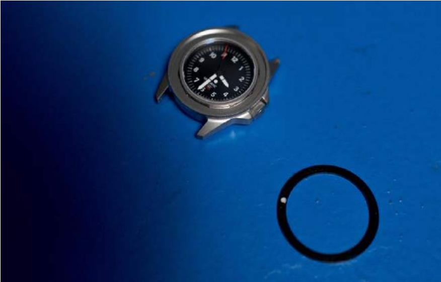
Figure 4 – Bezel insert detached.
