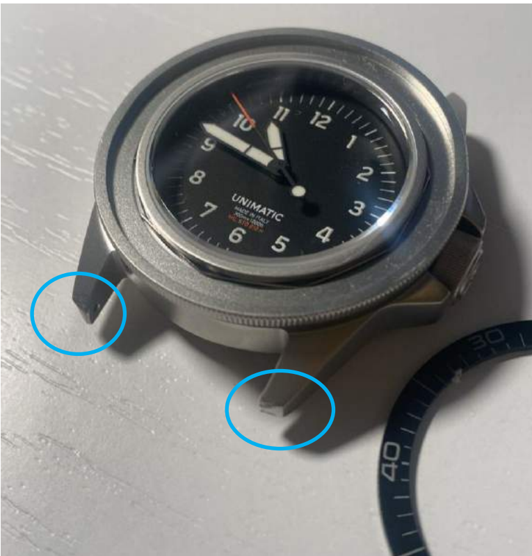
Figure 5 – Example of dents caused by the impacts
